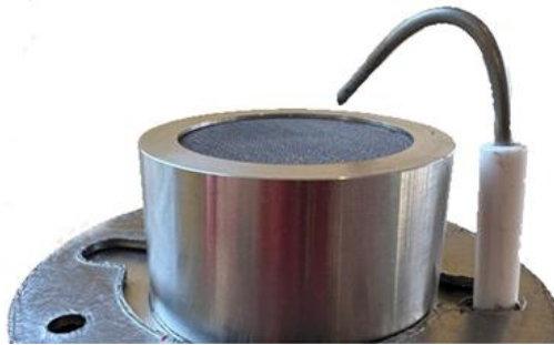
Figure 9: Positioning of the ignition electrode
